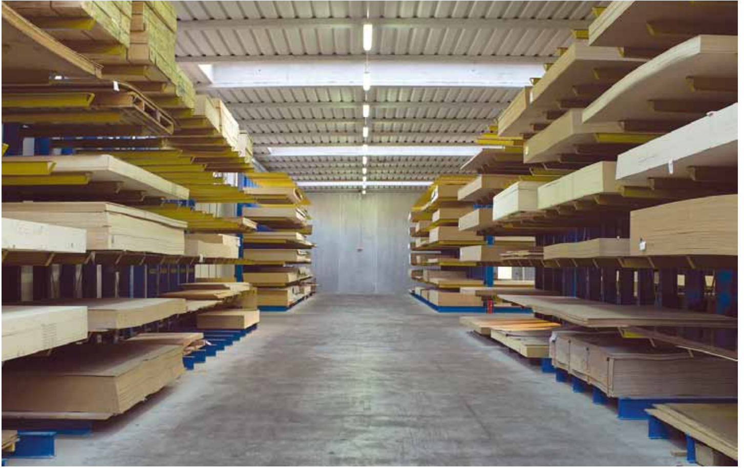
Cantilever a piano continuo, monofronte e bifronte
